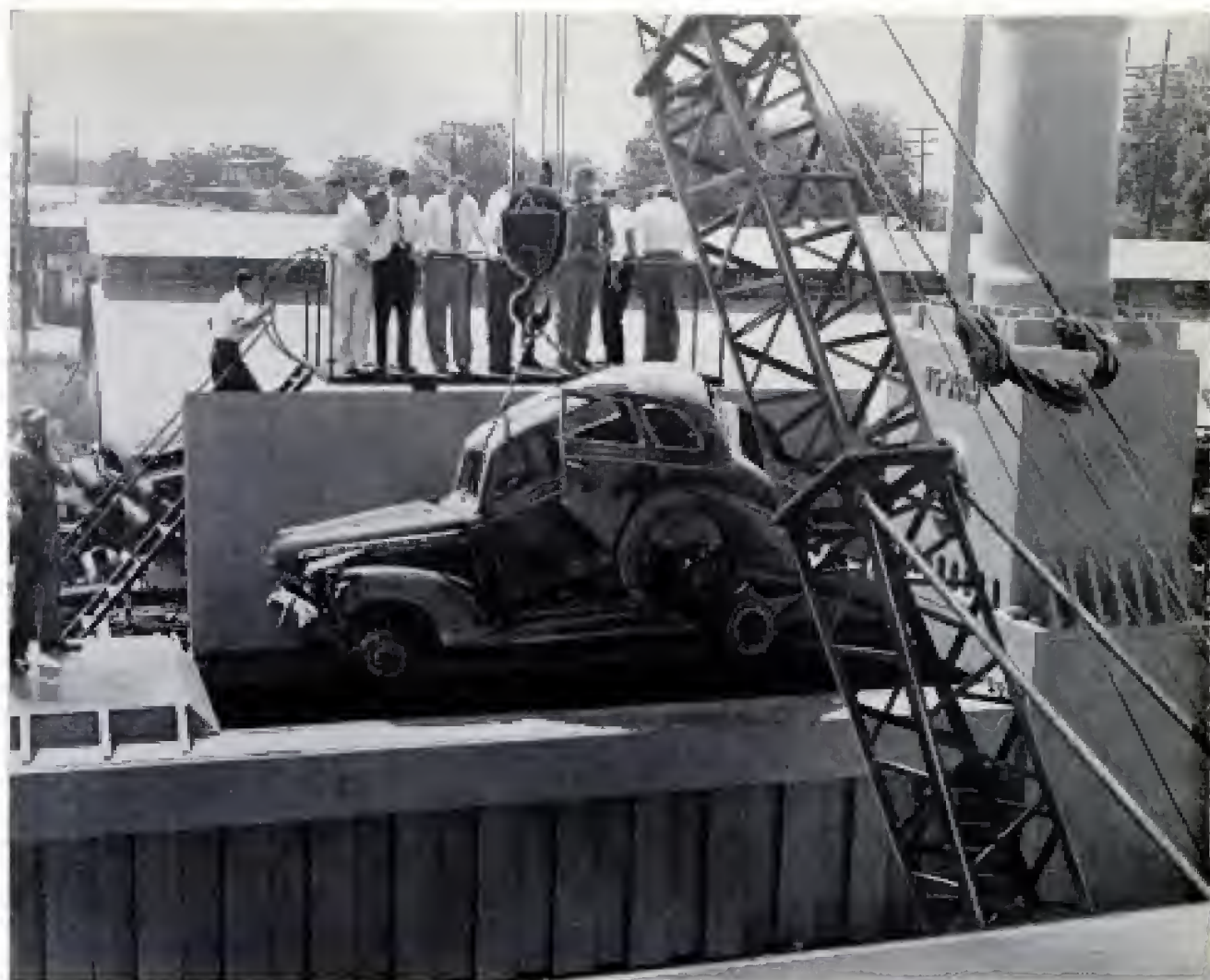
Old auto, engine and all, is dropped into the maw of the press. In seconds it will emerge as a little bale
